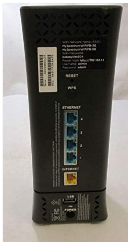
Figure 3.1: Rear panel of the Askey RAC2V1K router, displaying the power input, USB port, four Ethernet LAN ports, and one Internet (WAN) port, along with WPS and Reset buttons.
