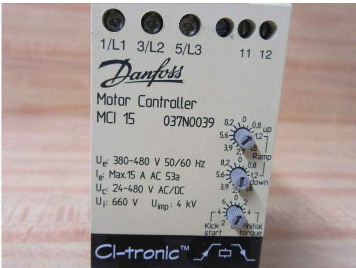
Figure 3.2: Close-up of the Danfoss MCI 15 Motor Controller's front panel, detailing the model number (MCI 15, 037N0039), electrical ratings, and adjustment potentiometers for ramp up, ramp down, kick start, and initial torque.
