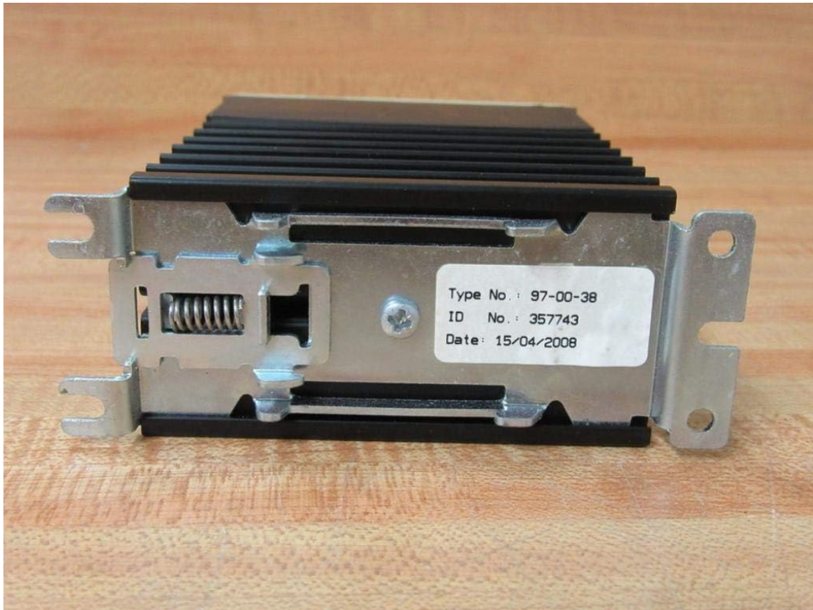
Figure 9.1: Rear view of the Danfoss MCI 15 Motor Controller, displaying a label with Type No., ID No., and Date of manufacture.
