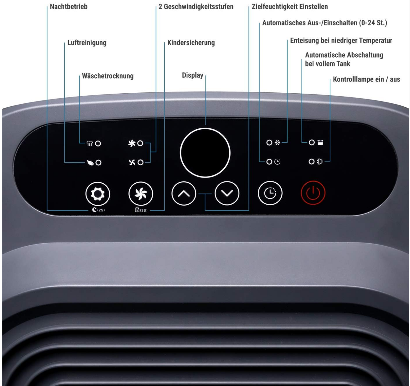
Figure 2: Detailed view of the Noaton DF 4214 control panel. This image indicates the functions of each button and display area, including night mode, fan speeds, humidity settings, timer, child lock, defrost, and water tank alerts.
