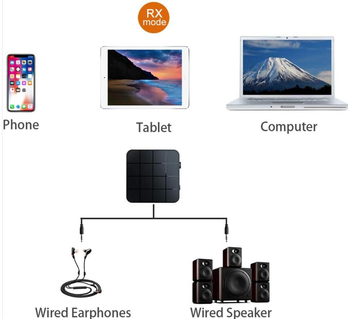
This diagram illustrates the adapter in Receiver (RX) mode, enabling a wired stereo system, speakers, or headphones to receive audio wirelessly from a Bluetooth-enabled phone, tablet, or computer.
