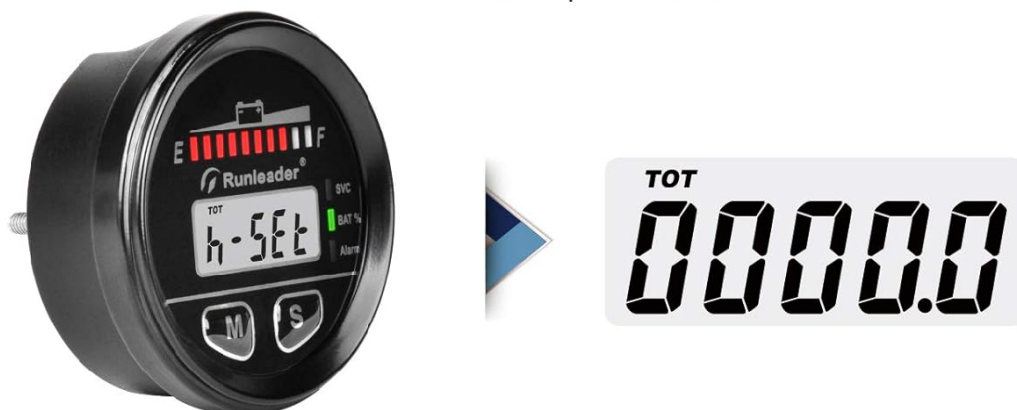
Figure 4.2.1: Display showing the Total Hour Meter (TOT) function.
