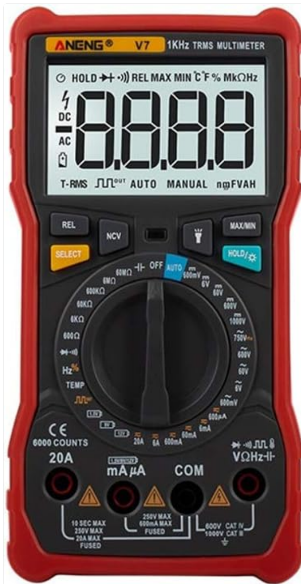
Figure 1.1: Front view of the ANENG V7 Digital Multimeter, showcasing its display, rotary dial, and input jacks.
