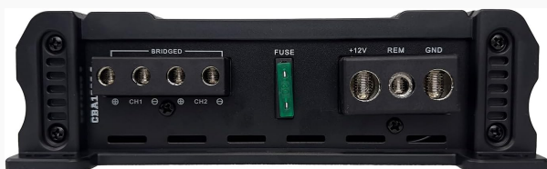
Figure 2: Rear view of the amplifier, showing the power, ground, remote, and speaker output terminals, along with the fuse.
