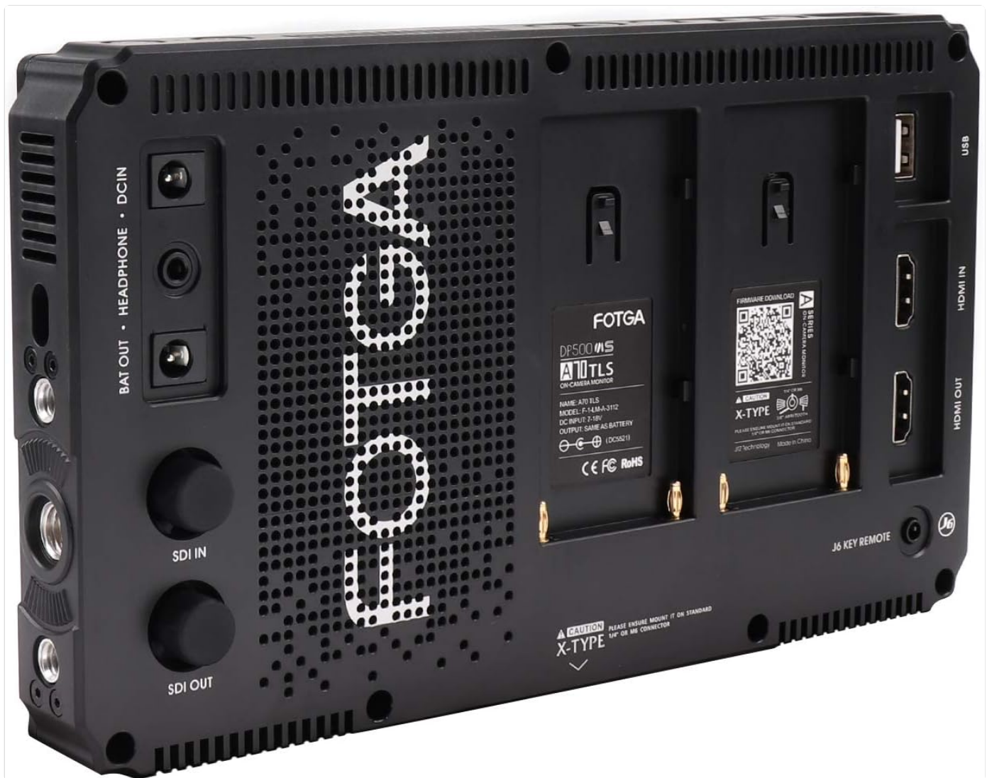
Figure 2.2.2: Rear panel of the monitor. This view highlights the dual NP-F battery plates, HDMI input/output, SDI input/output, USB port, and DC power input, along with the headphone and battery output ports.
