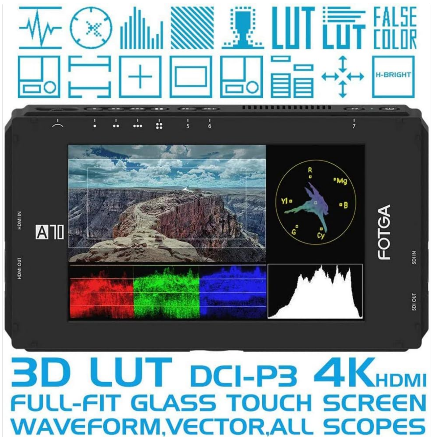
Figure 3.2.1: Advanced monitoring tools. This image illustrates the monitor's capability to display 3D LUTs, waveform, vector scope, and other professional analysis tools simultaneously, aiding in precise image evaluation.
