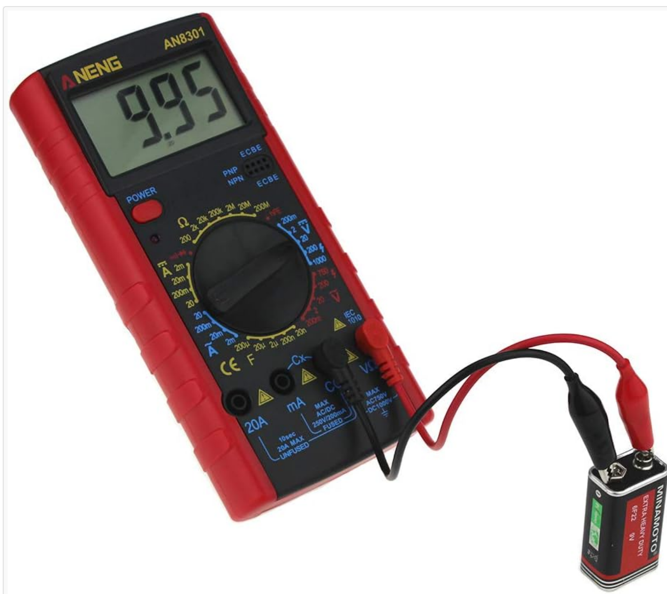
Figure 5.1: The ANENG AN8301 Multimeter displaying a voltage reading while connected to a 9V battery using test clips.
