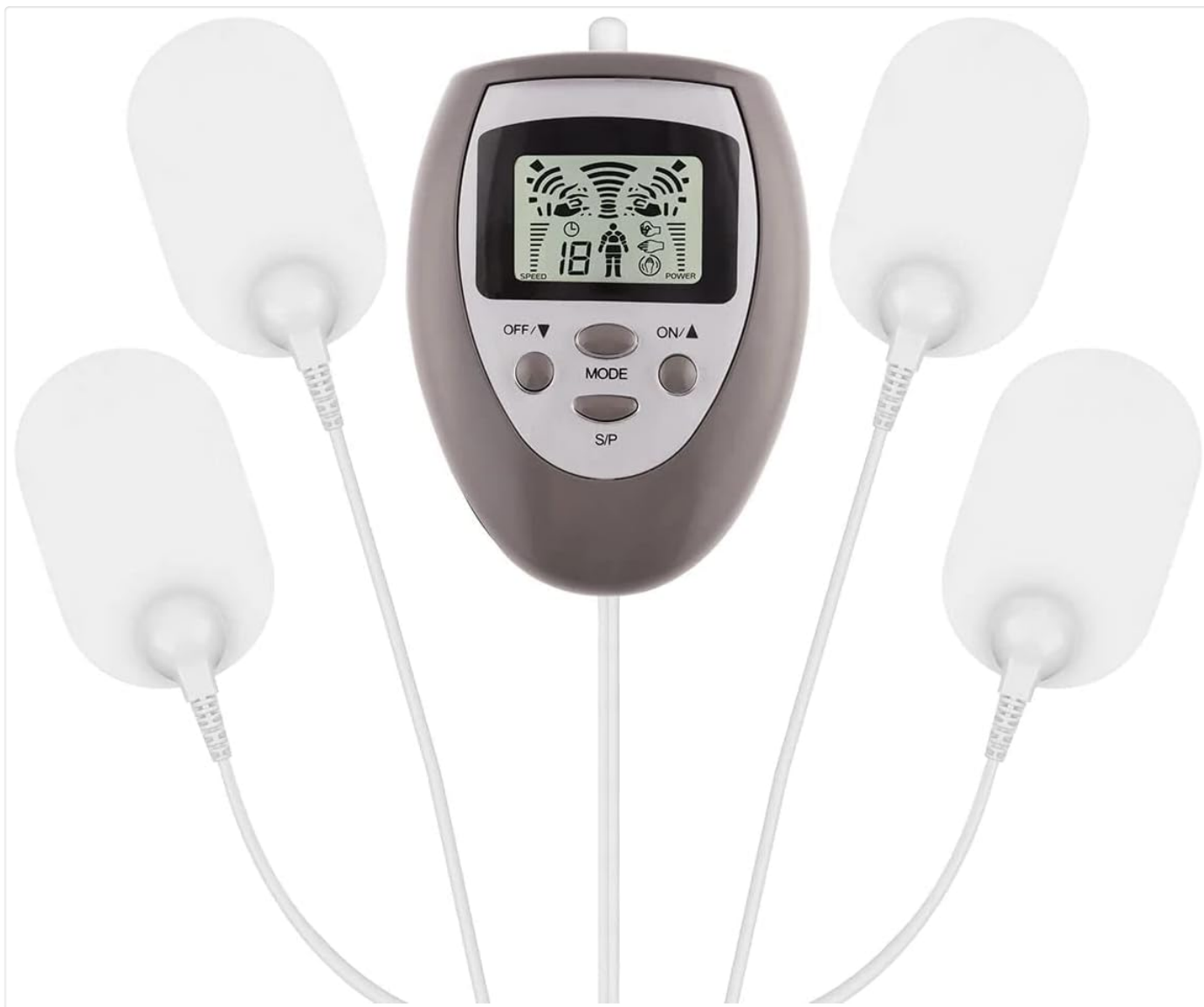
Image 4.1: The TENS electrostimulator unit with all four electrodes attached.
