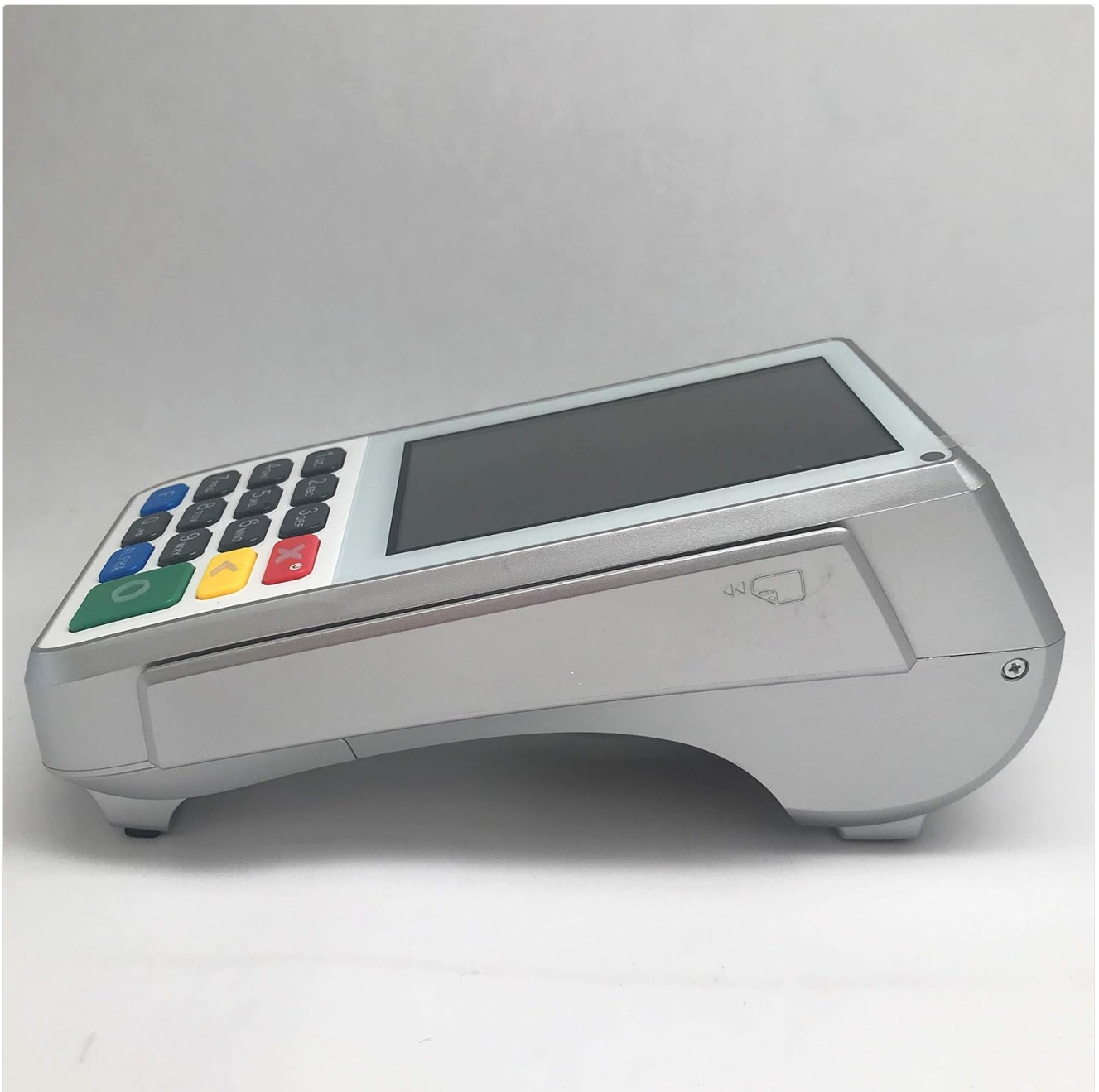
Figure 2.2.3: Side view of the PAX A80 terminal, highlighting the integrated magnetic stripe card reader slot on the right side of the device.
