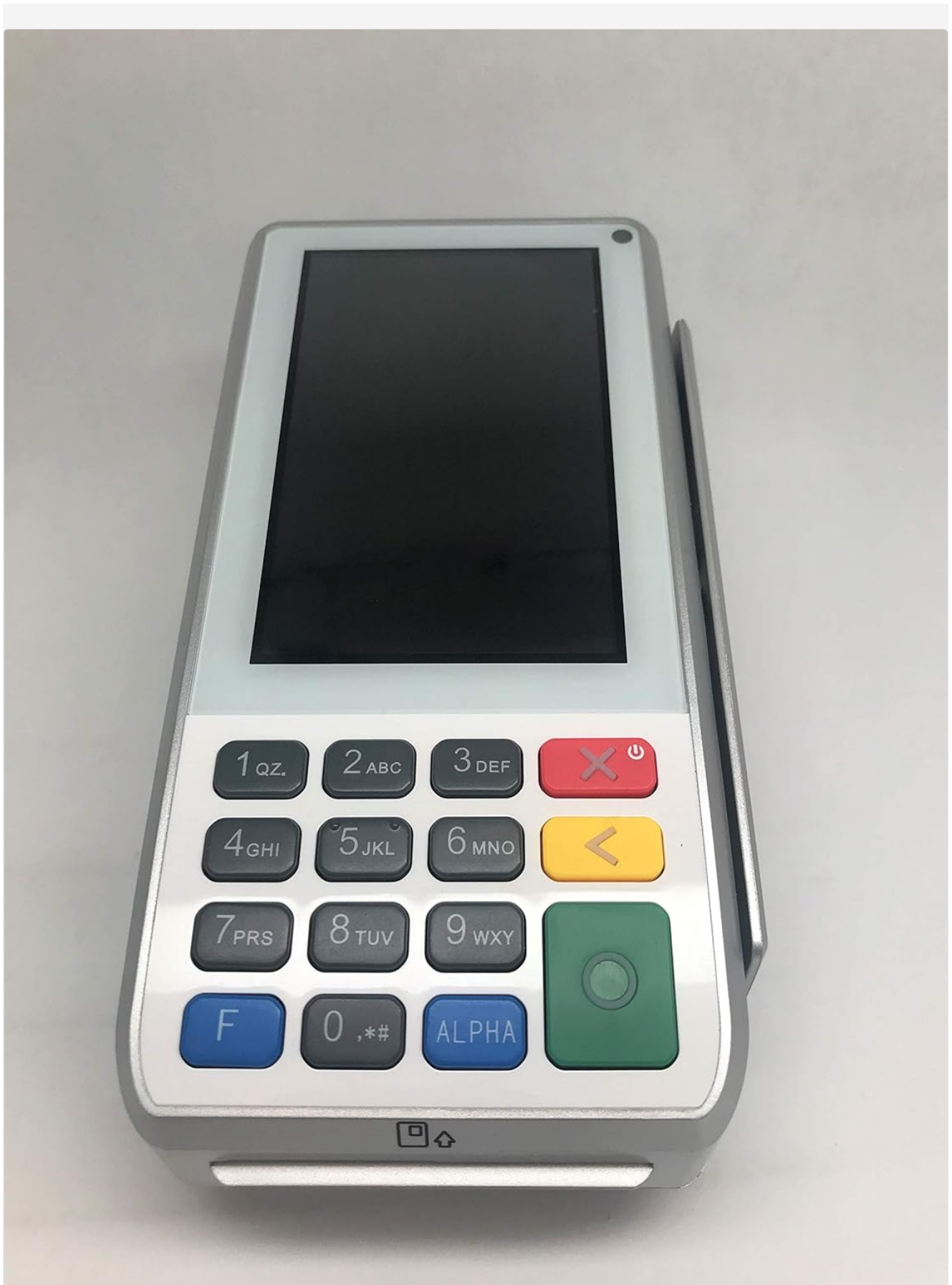
Figure 2.2.2: Angled front view of the PAX A80 terminal, providing a clear perspective of the device's overall design, the blank touchscreen, and the full keypad layout.
