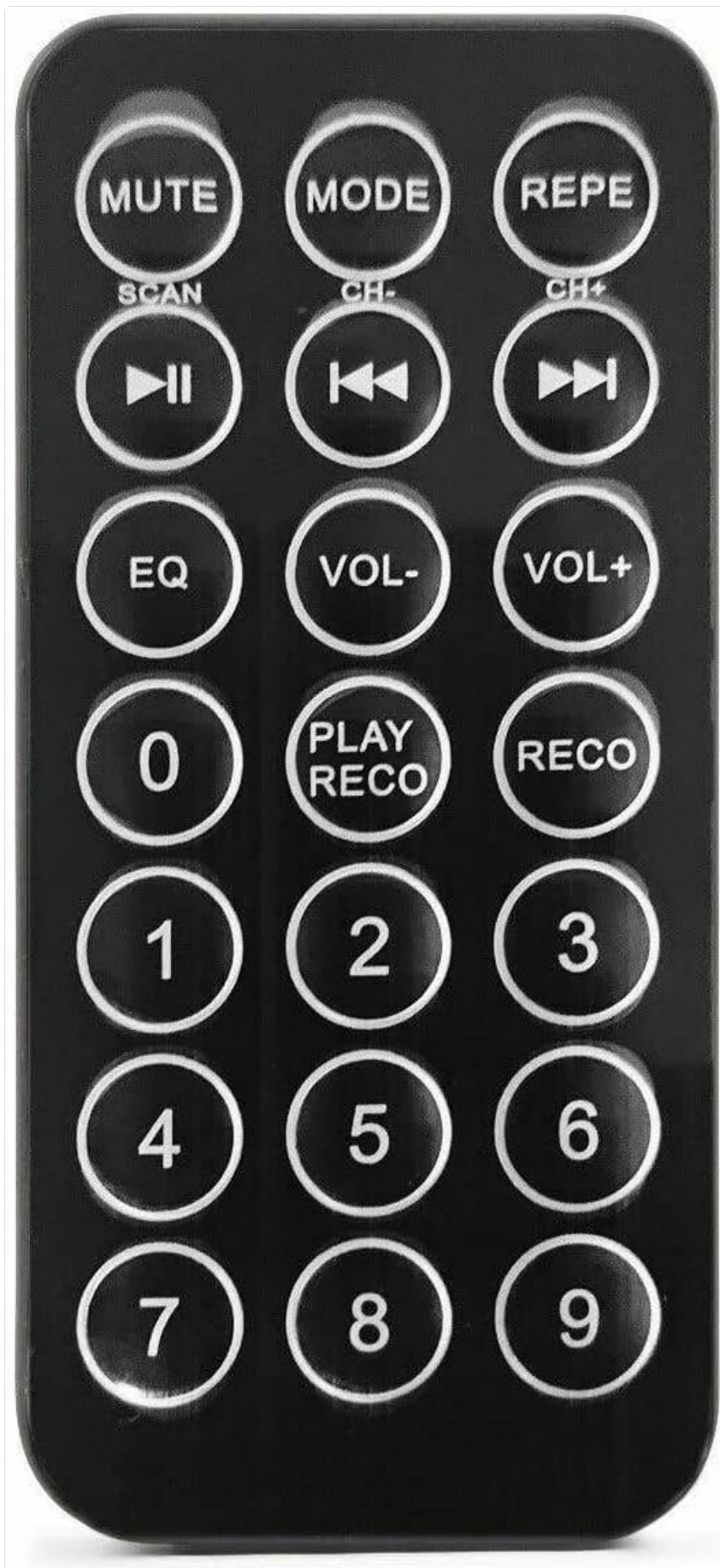
Image: The remote control for the FPC8T speaker, showing buttons for mute, mode, repeat, track control, volume adjustment, EQ, and numeric input.
