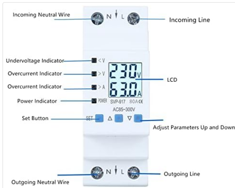
Figure 1: Front view of the Walfront Voltage Protector, highlighting the LCD display, undervoltage, overvoltage, and overcurrent indicators, as well as the 'SET' and adjustment buttons.
