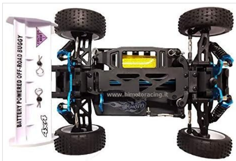
Image 3: Top-down view of the Himoto EXB-16 chassis, showing the layout for electronic components and the central drive shaft.
