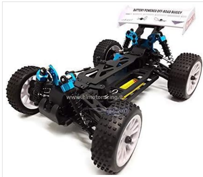
Image 2: Side view of the Himoto EXB-16 chassis, highlighting the suspension and drive train components.
