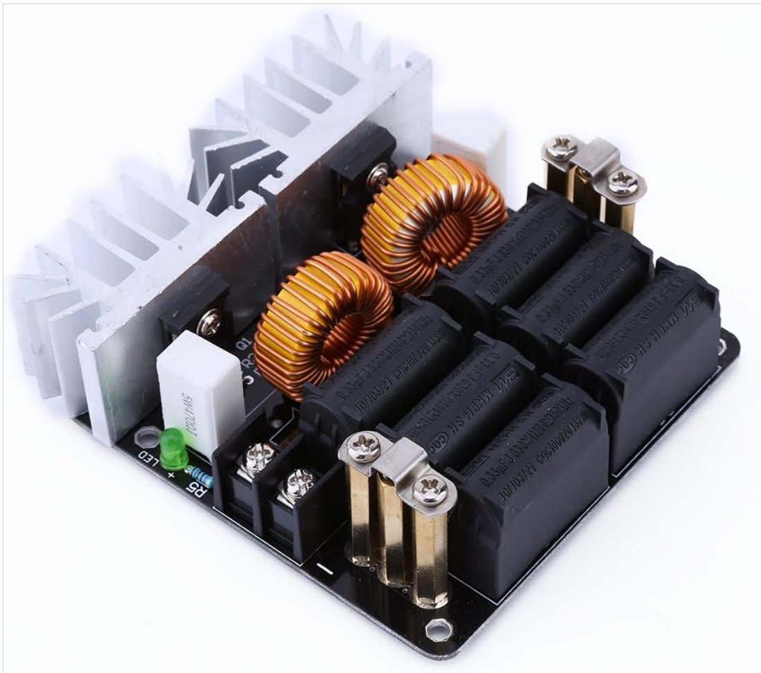
Image 5.2: Top view of the ZVS module, showing connection points and components.
