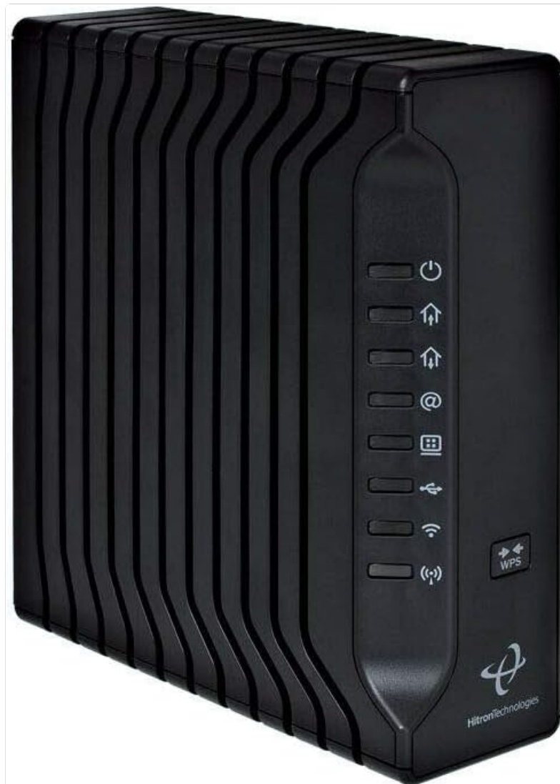
Figure 4.1: Front view of the Hitron CGN Wireless Gateway Modem Router. This image shows the vertical orientation of the device with a ribbed design on the left and a smooth panel on the right containing LED indicators and a WPS button.
