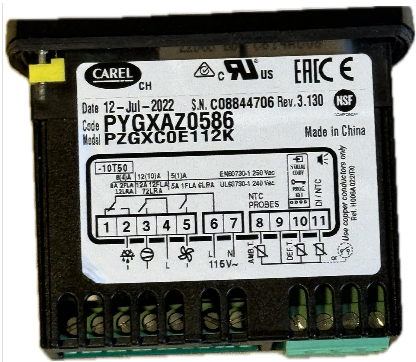
Image: The top view of the Carel thermostat, displaying the detailed wiring diagram and model information on its label.
