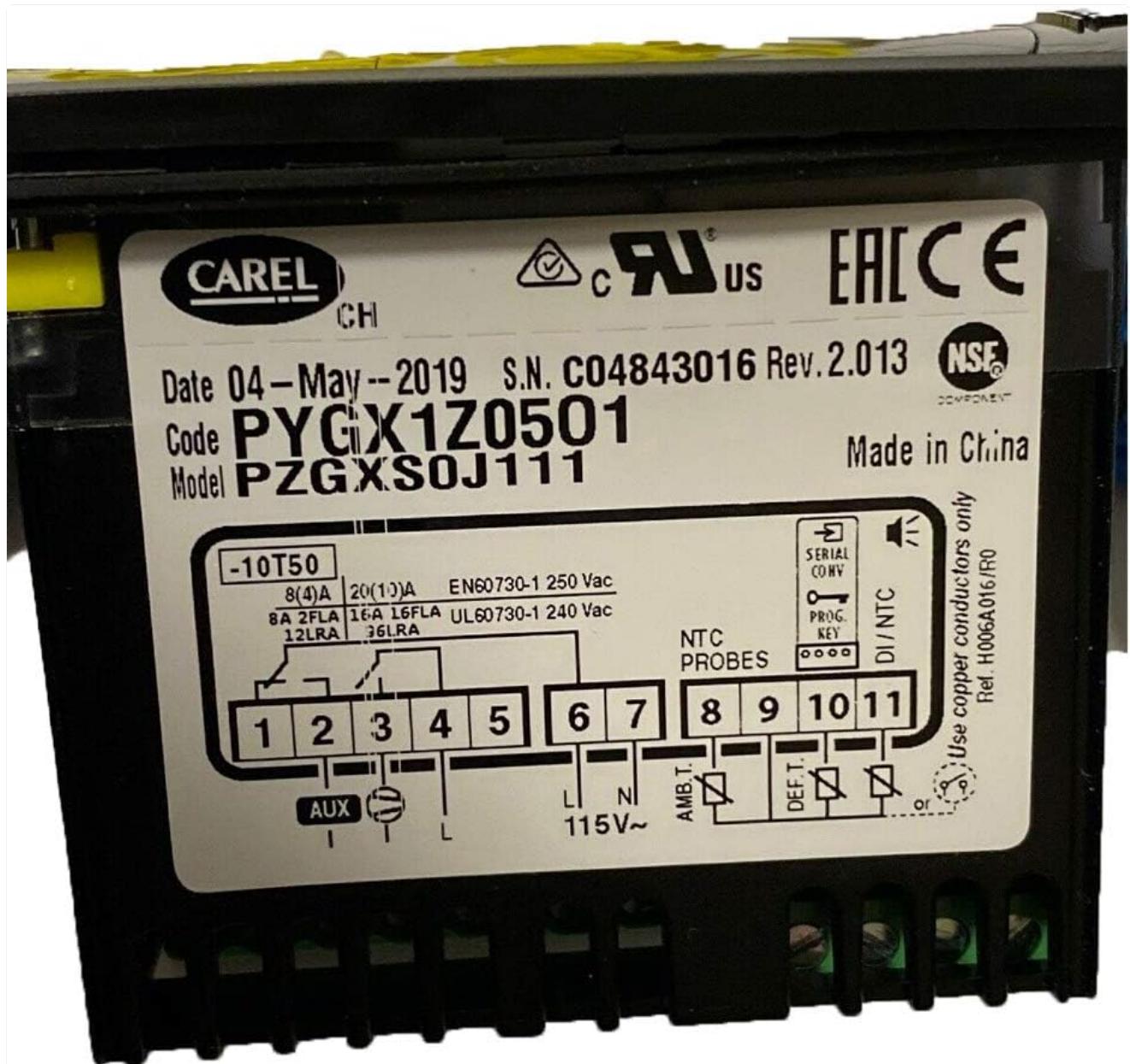
Image 2: Rear view of the thermostat, displaying the wiring diagram and terminal connections.
