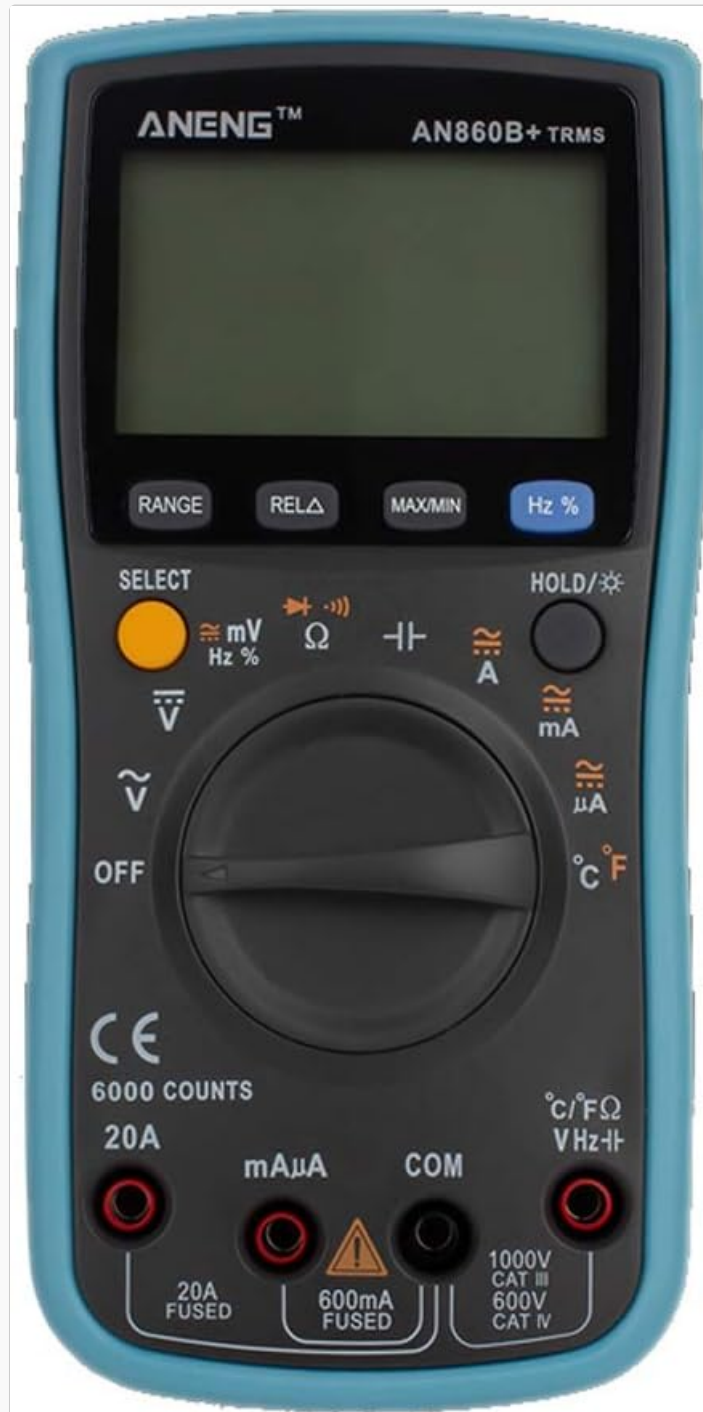
Figure 1: Front view of the ANENG AN860B+ Digital Multimeter, showing the display, function dial, and input jacks.
