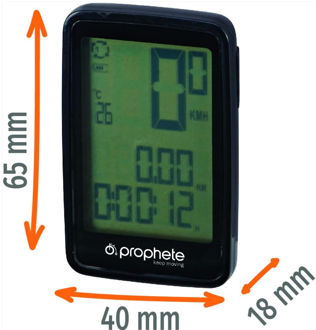
Image 2: Dimensions of the Prophete Bicycle Computer. The image shows the device measuring approximately 65 mm in height, 40 mm in width, and 18 mm in depth.
