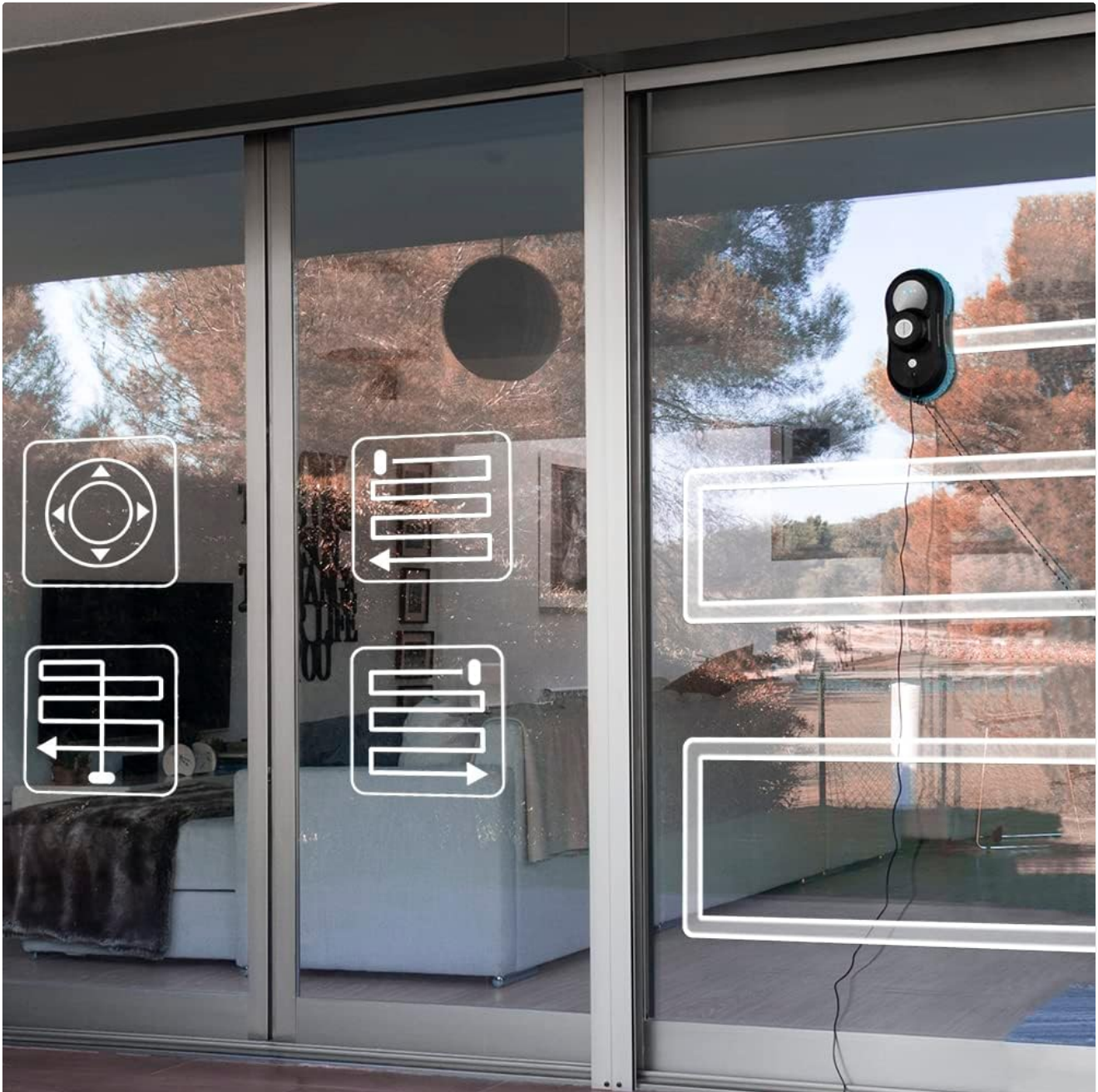
Figure 5.2: Visual representation of the robot's intelligent cleaning paths, including Z-path, N-path, and manual control options, demonstrating its navigation capabilities.
