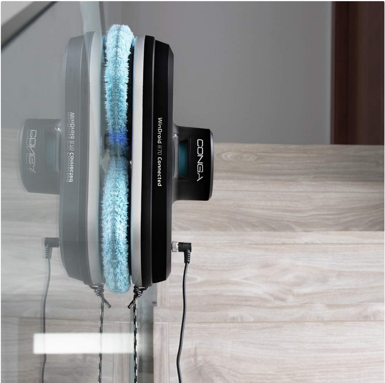
Figure 2.1: The robot securely attached to a window, demonstrating the proper connection of the power cable and the safety rope for secure operation.
