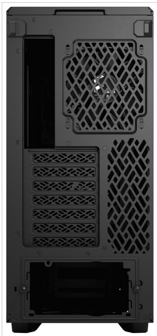
Rear view of the case, showing the exhaust fan mount and PCIe slots.
