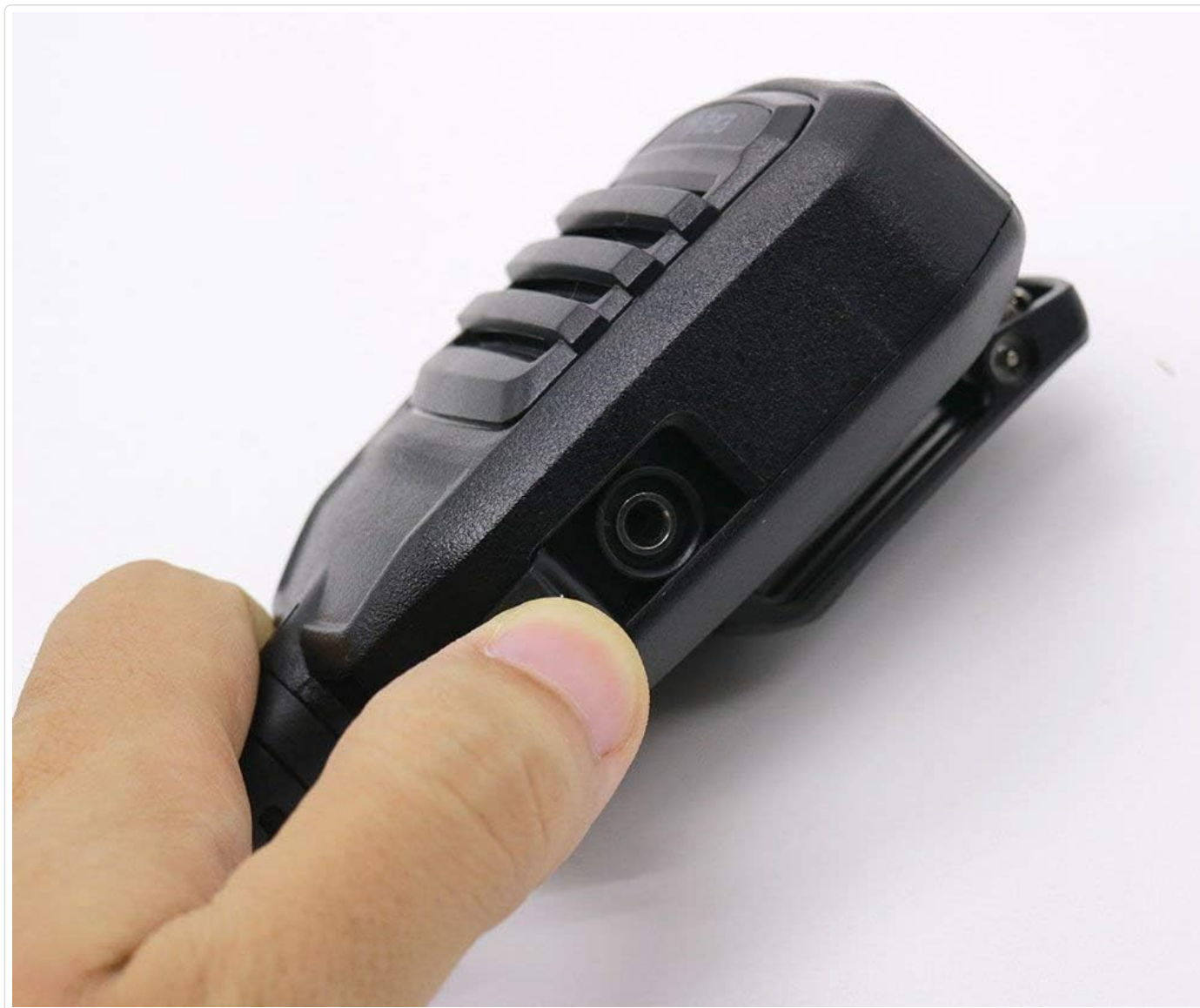
Figure 5: A hand demonstrating the position of the 3.5mm audio jack on the side of the microphone, used for connecting an earpiece.
