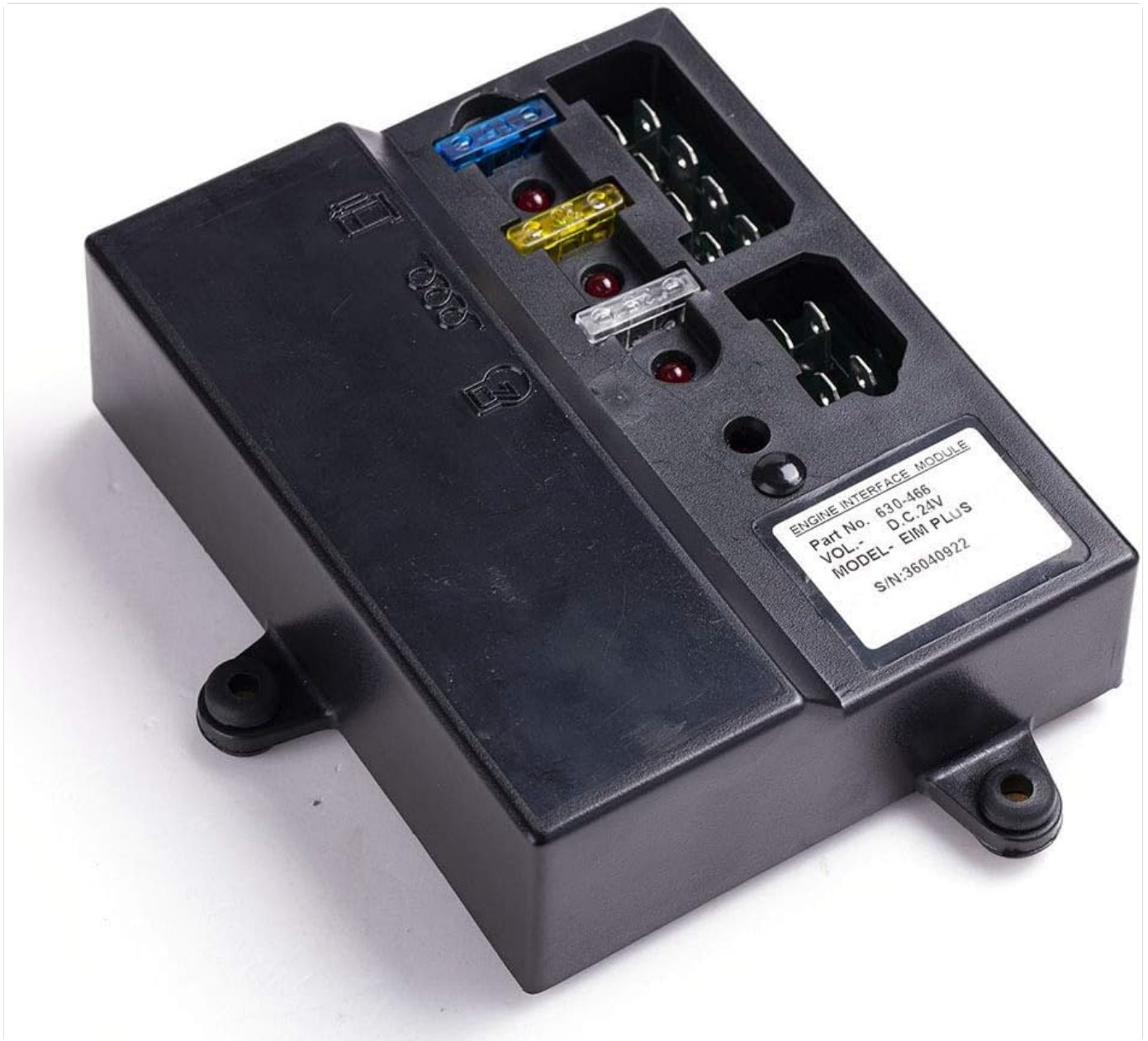
Image 4.1: Angled view of the Knowtek EIM Plus 630-466 module, illustrating its side profile and the integrated mounting tabs. This perspective is useful for understanding how the module can be secured during installation.
