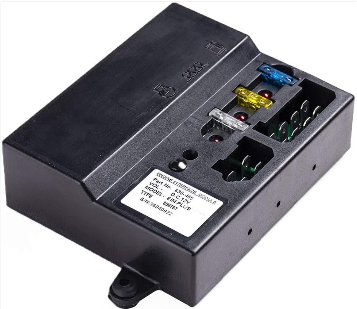
Figure 1: Knowtek Engine Interface Module EIM PLUS 630-465, showing its compact design and integrated fuses.
