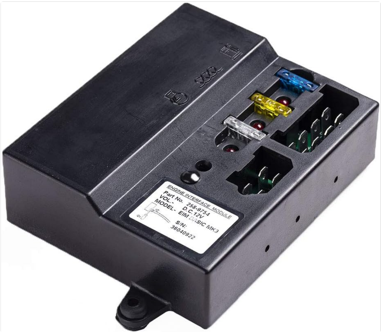
Figure 1.1: Front view of the Knowtek EIM Basic MK3 module, showing the label with part number and model, along with fuse slots and connection points.
