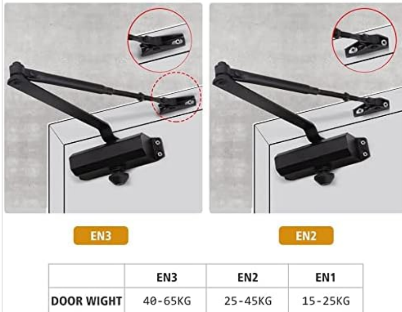
Image: Diagram showing how adjusting the arm shoe position affects the closing power (EN3 for 40-65KG, EN2 for 25-45KG, EN1 for 15-25KG).
