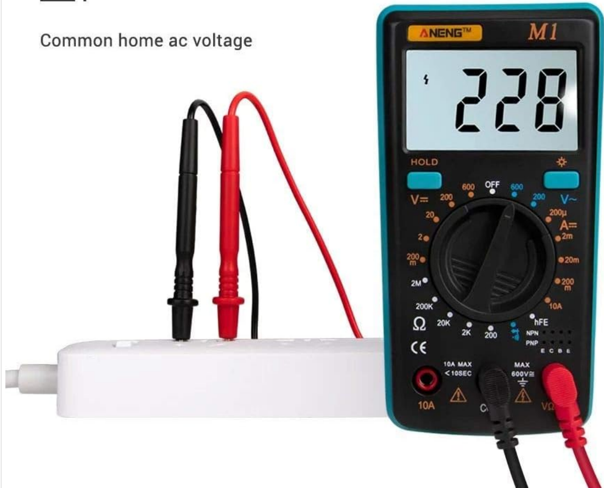
Figure 5.1: The ANENG M1 multimeter measuring AC voltage from a standard wall outlet, demonstrating proper test lead connection.
