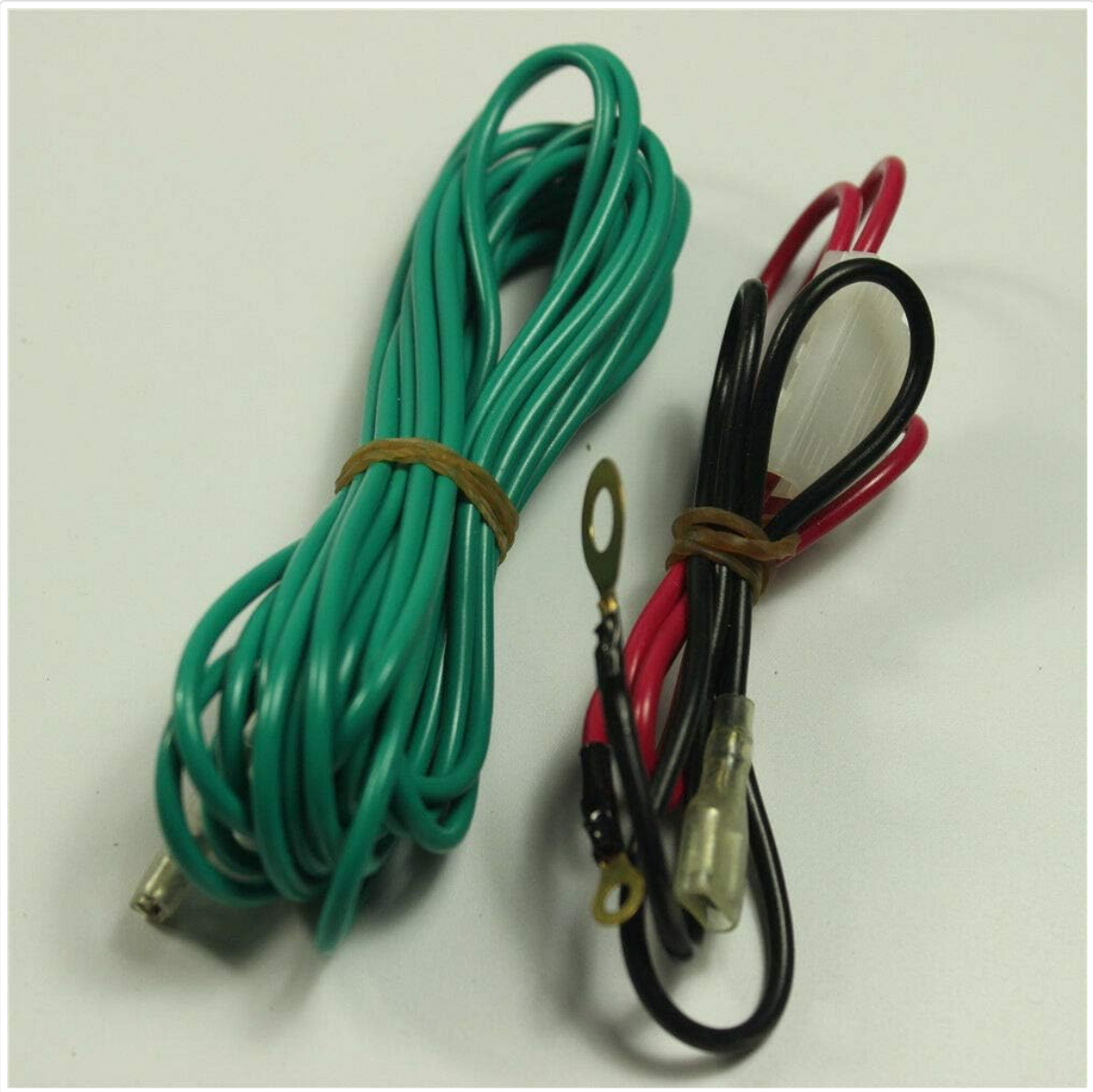
Image: Bundles of green and red/black electrical wires with terminal connectors, used for various connections within the kit.
