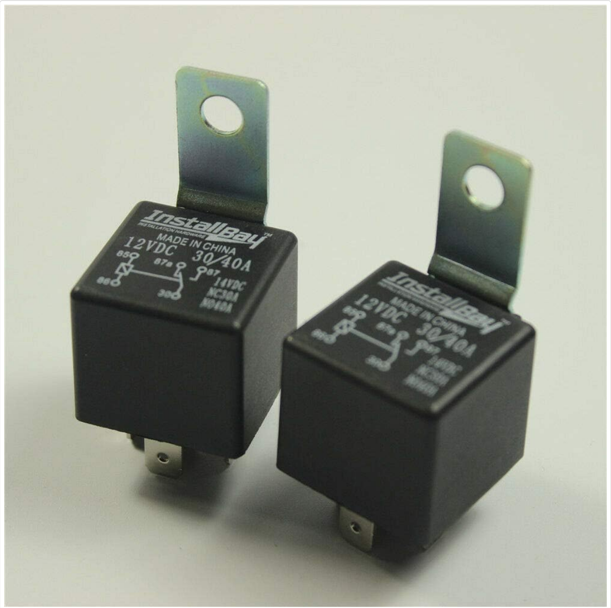
Image: Two 12VDC 30/40A automotive relays, essential for controlling the solenoids.
