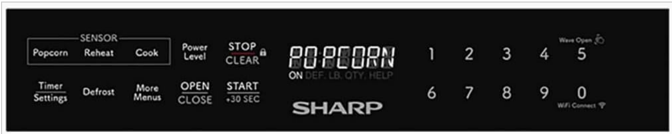
Figure 4: Close-up view of the concealed glass touch control panel.
