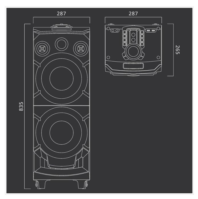
This technical drawing provides precise measurements of the Muse M-1935 DJ speaker, indicating its height (835mm), width (287mm), and depth (265mm). These dimensions are crucial for planning placement and transportation.
