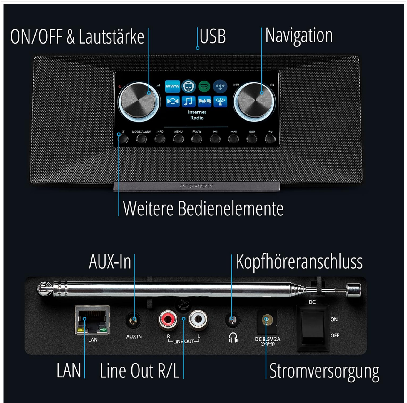
Figure 4.2: Labeled diagram showing the front panel controls (ON/OFF & Volume knob, USB port, Navigation knob, Mode/Alarm, Info, Menu, Favorites, Play/Pause, Skip, Back buttons) and rear panel ports (LAN, AUX In, Line Out R/L, Headphone Jack, DC 9V 2A Power Supply, ON/OFF switch).
