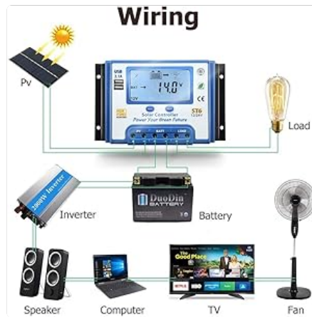
Figure 4: Wiring diagram illustrating connections for solar panel, battery, and load to the SolaMr Solar Charge Controller, including an optional inverter.
