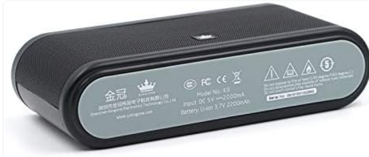
Image 7.1: Speaker Bottom Panel. This image shows the bottom panel of the KINGONE K9 speaker, displaying regulatory marks, model number, input voltage, and battery specifications.
