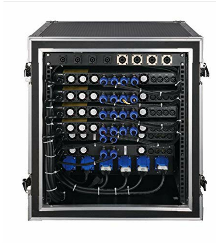
Figure 3.3: Detailed rear view of multiple CVR D-Series amplifiers within a rack, illustrating typical cabling for professional setups.
