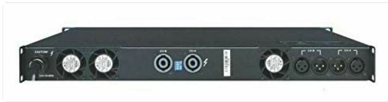
Figure 3.2: Rear panel of the CVR D-802 amplifier, highlighting the XLR input, Speakon output, and power connections.
