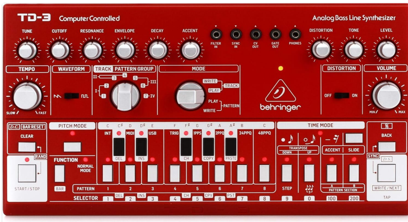
Figure 1: Front view of the Behringer TD-3-RD Analog Bass Line Synthesizer, showing controls for tune, cutoff, resonance, envelope, decay, accent, distortion, volume, and the 16-step sequencer interface.
