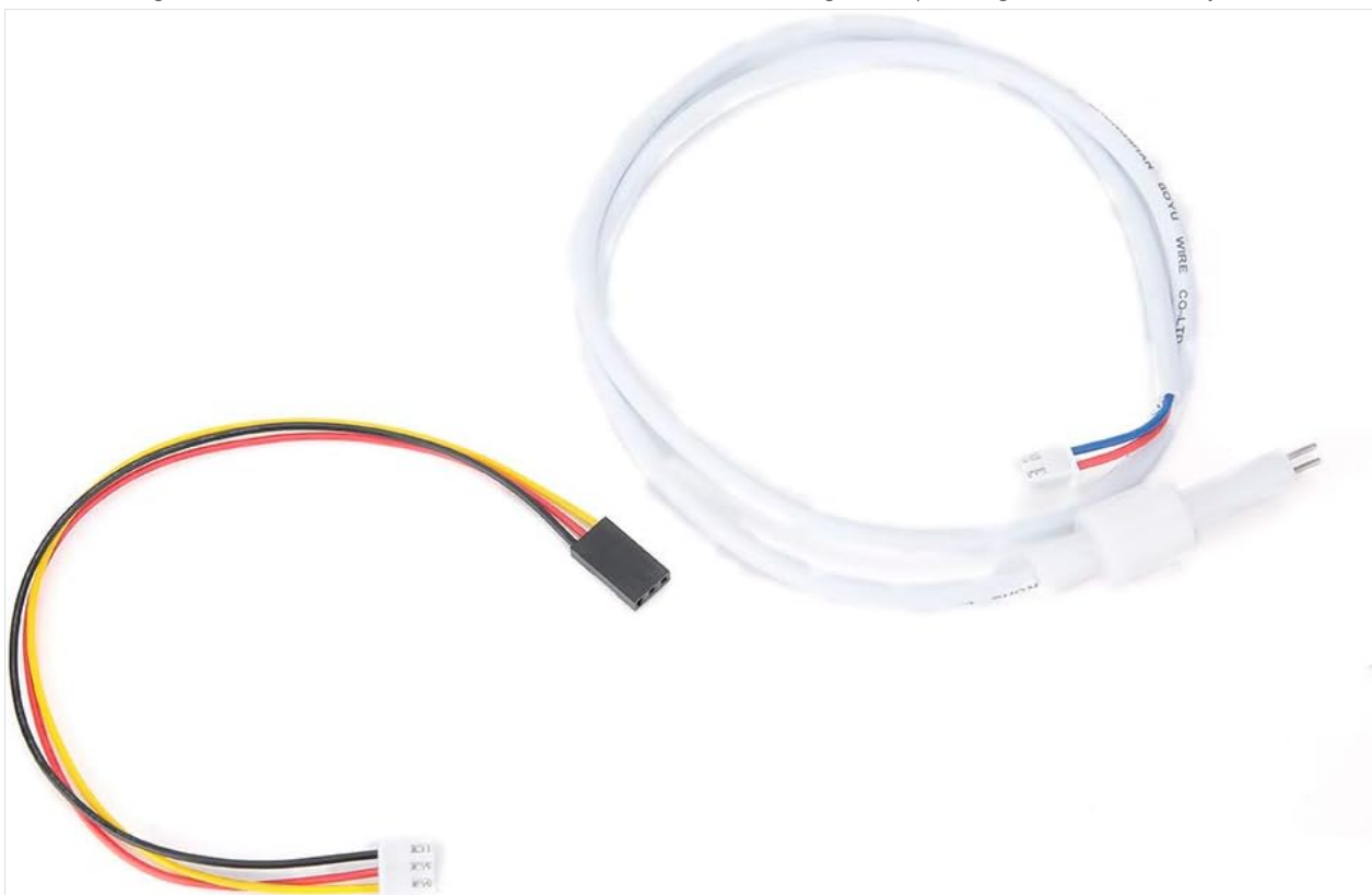
Image: Close-up view of the connection cables for the ASHATA TDS sensor, showing the XH2.54-3P and XH2.54-2P connectors.
