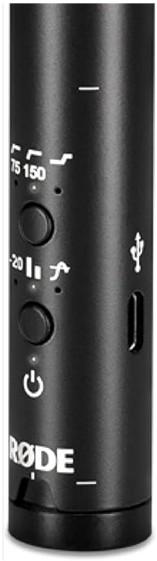
Figure 2: Side view of the Rode VideoMic NTG, highlighting the control buttons for gain, high-pass filter, -20dB pad, high frequency boost, and the USB-C port for charging and digital audio output.
