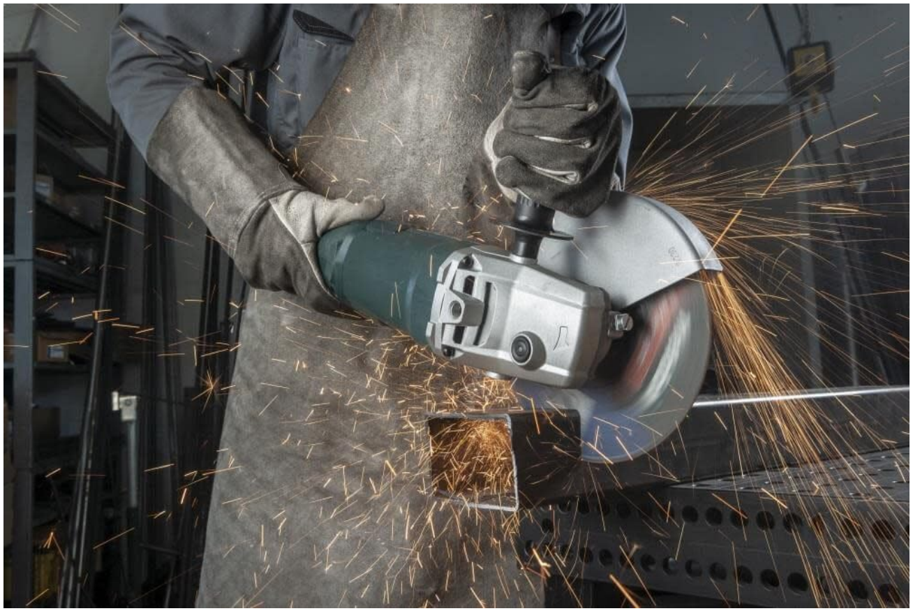
Figure 3: Angle Grinder in Operation
