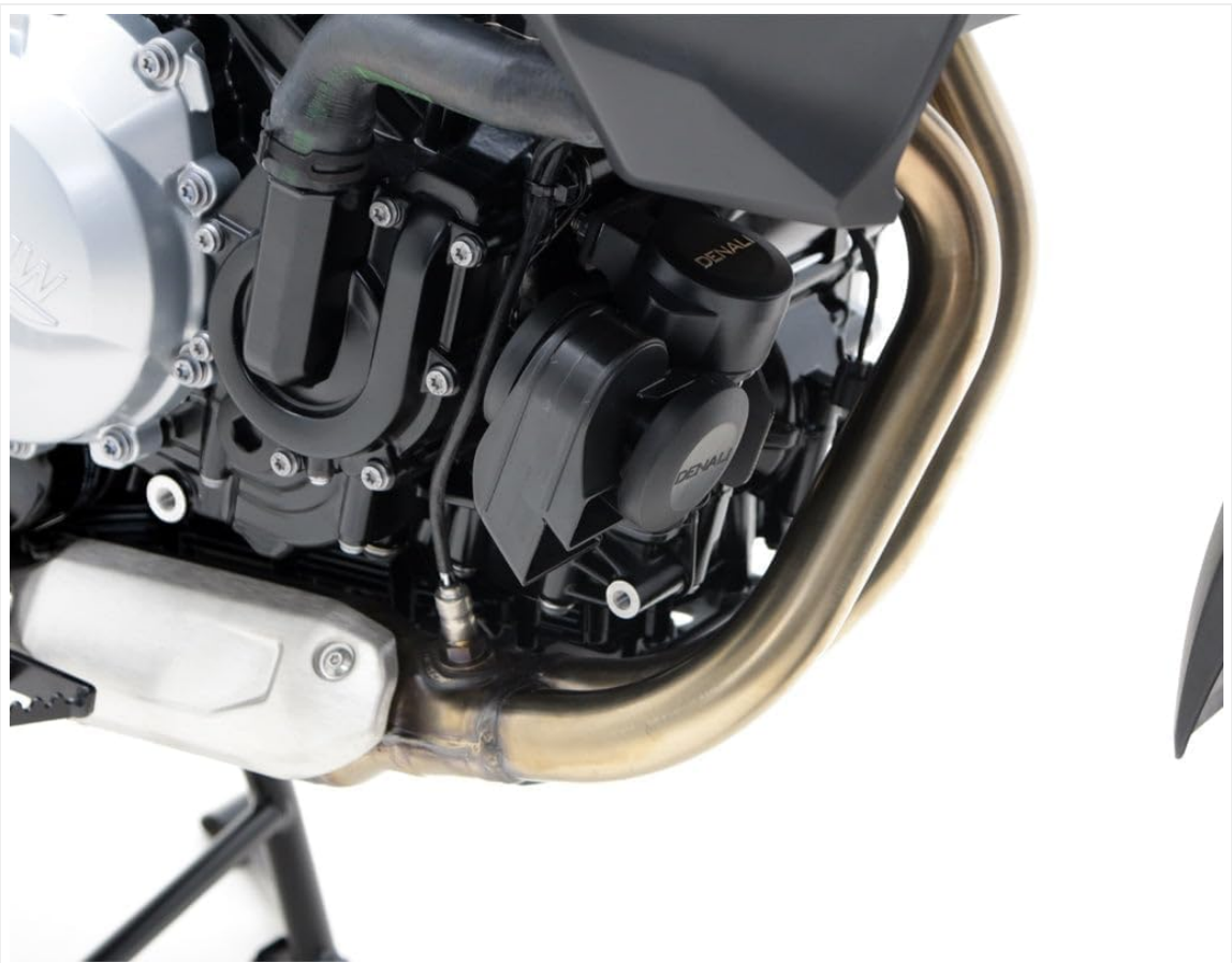
Image: The DENALI horn mount bracket securely attached to the motorcycle engine, ready for horn installation.
