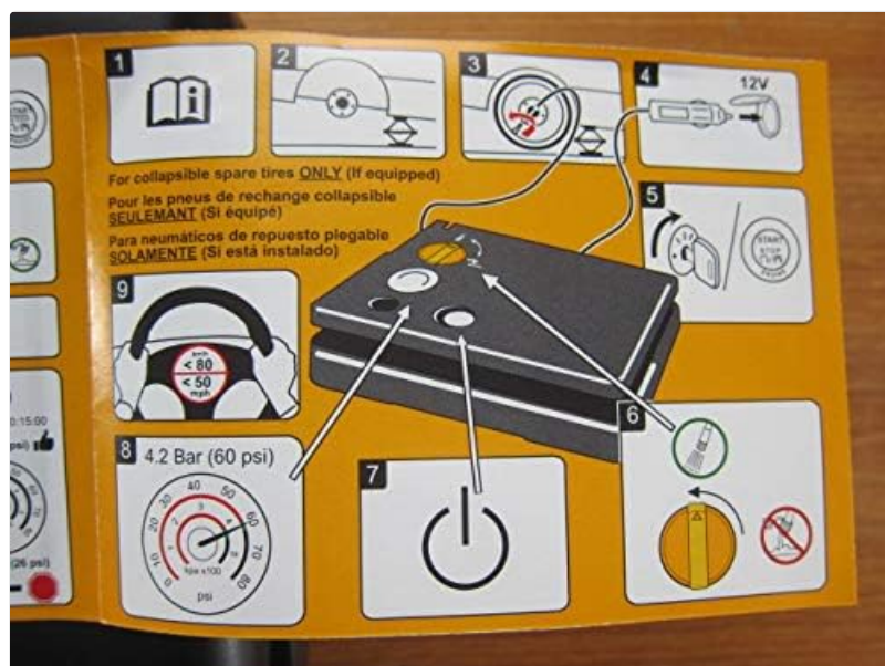
Image: Step-by-step visual instructions for inflating a collapsible spare tire.
