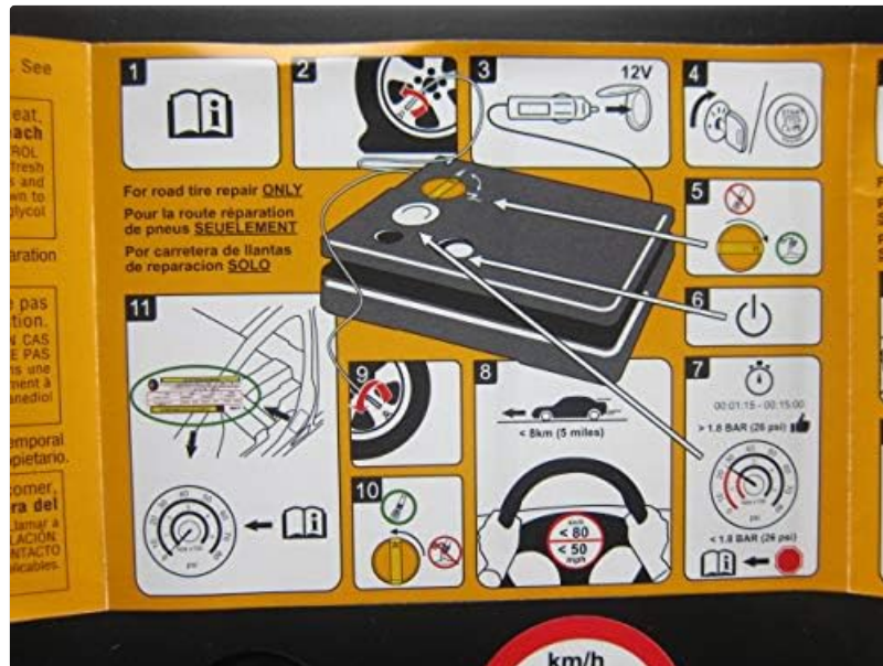
Image: Step-by-step visual instructions for temporary road tire repair.
