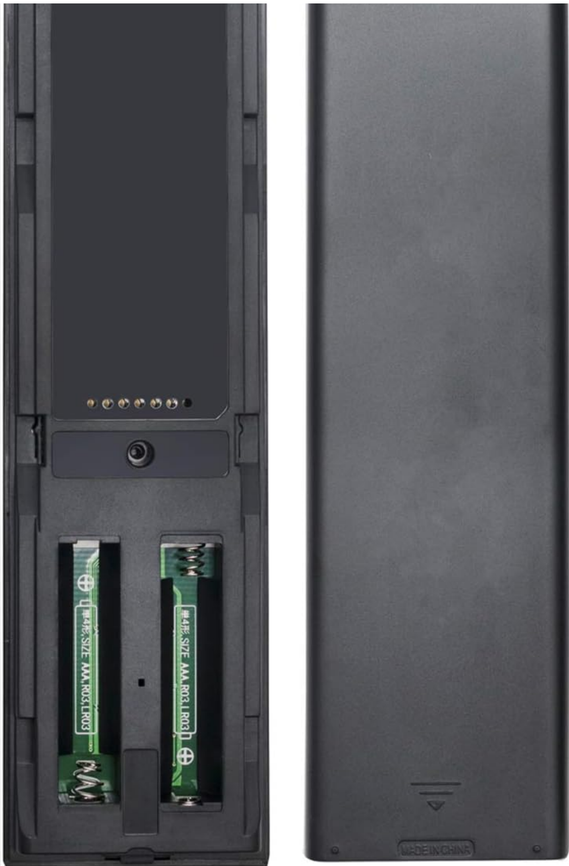
Image: Back view of the ALLIMITY RMF-TX310U Voice Remote Control, showing the open battery compartment with slots for two AAA batteries.
