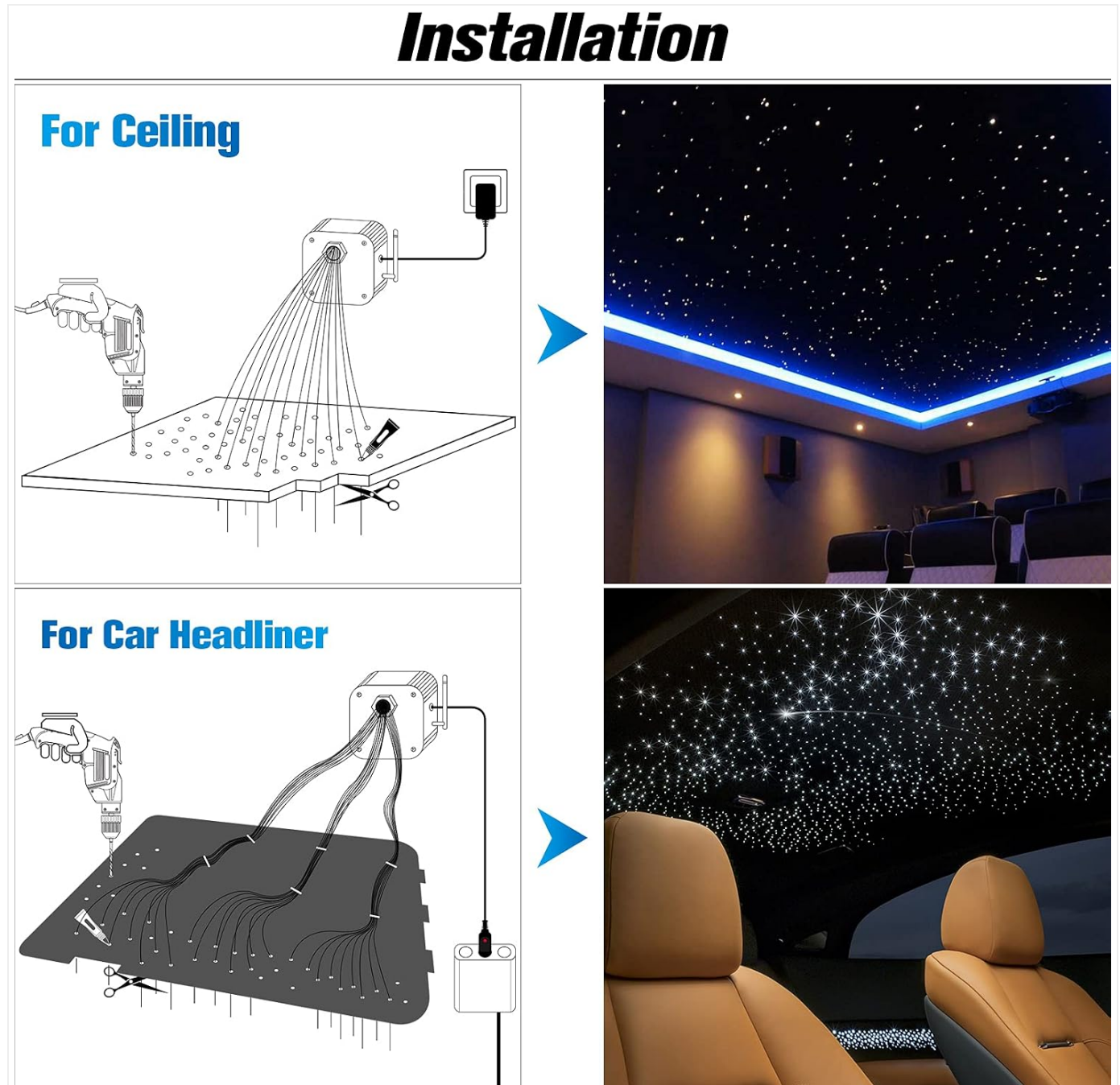
Image 3.2: Installation diagrams for ceiling and car headliner applications.
