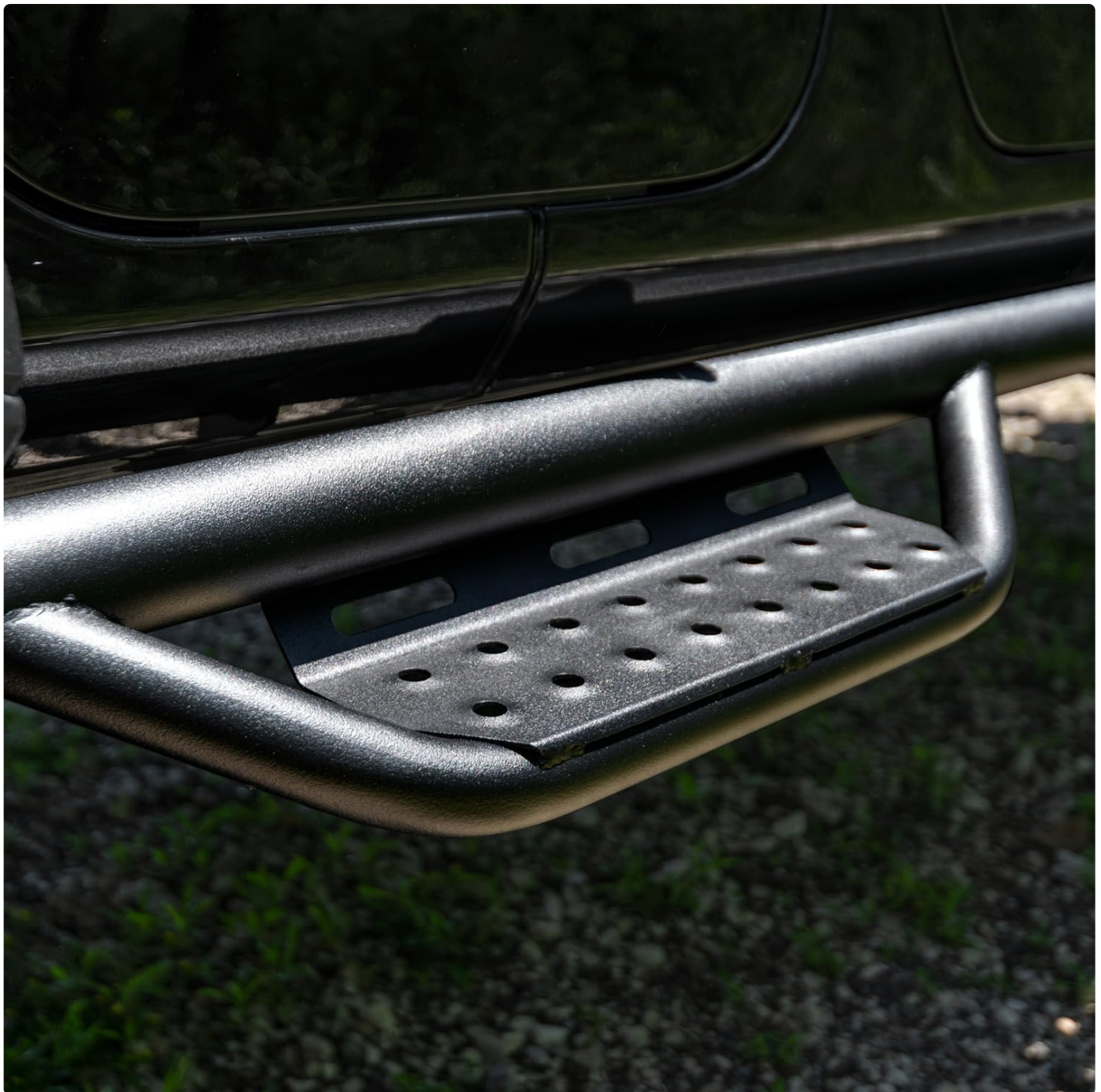
Image: Close-up of the textured step surface, designed for enhanced grip and stability.
