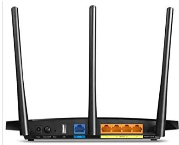
Figure 3.3: Rear view of the TP-Link Archer C90 router. This image clearly shows the various ports and buttons located on the back of the router, including the power input, power on/off switch, USB ports, WAN port (blue), and four Gigabit LAN ports (yellow). Also visible are the WPS/Reset button and the Wi-Fi on/off button.
