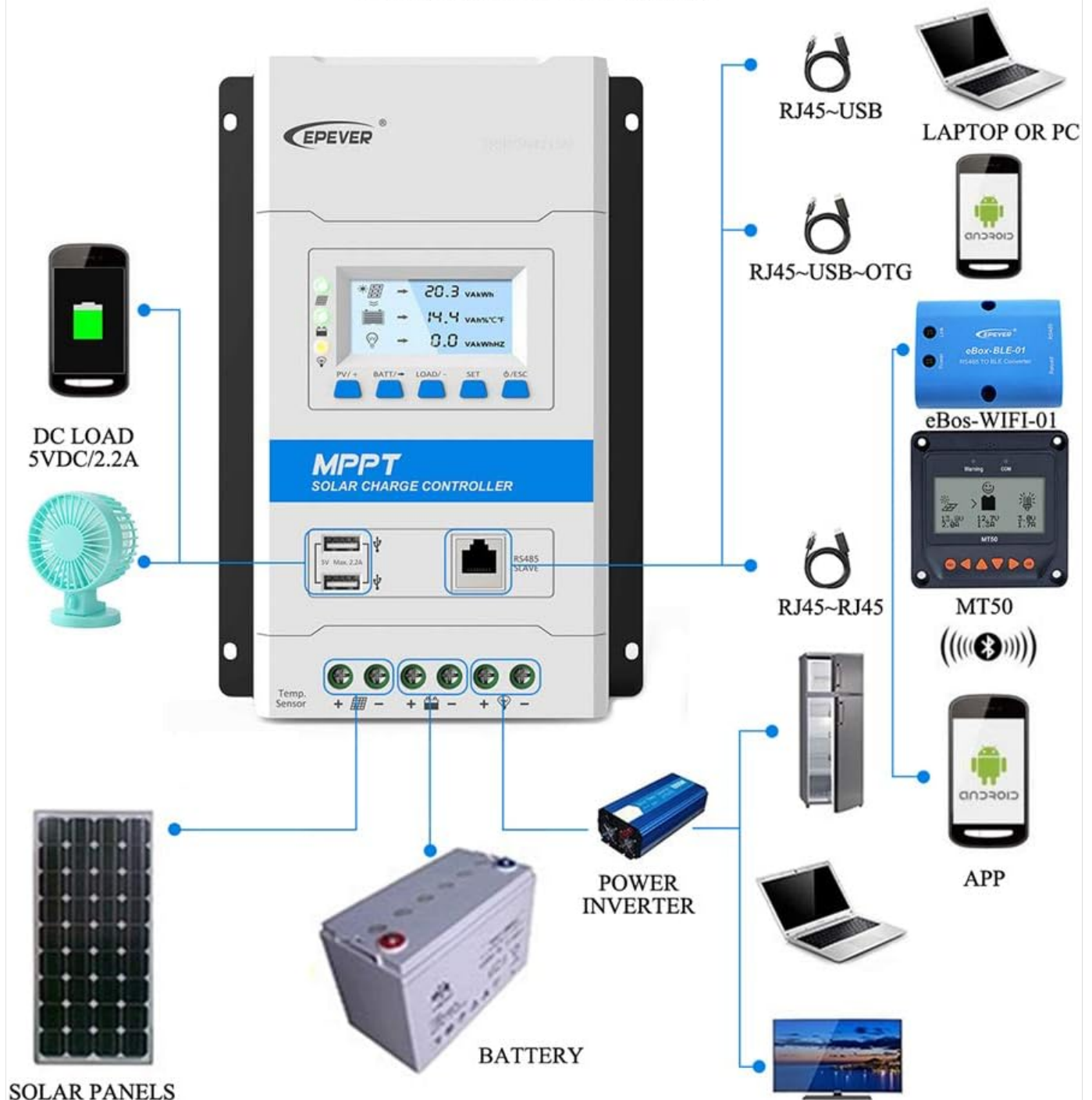
Figure 5: System connection diagram for the EPEVER TRIRON 4210N controller.
