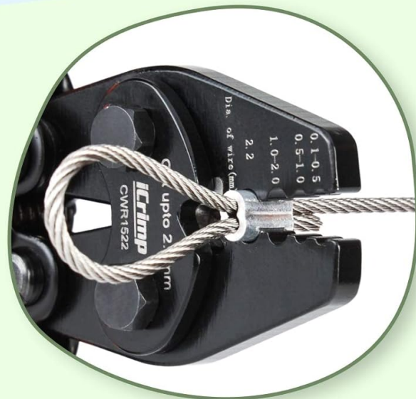
Image 6.2: Visual guide for cutting wire rope and crimping oval sleeves.
