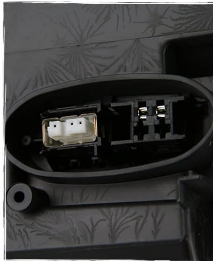
Figure 2: Rear view of the headlight assembly, showing the various electrical connectors and mounting points. Ensure all connections are firm.
