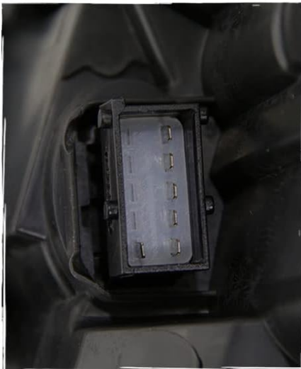
Figure 2: Rear view of the headlight assembly, showing the various electrical connectors and mounting points. Ensure all connections are firm.
