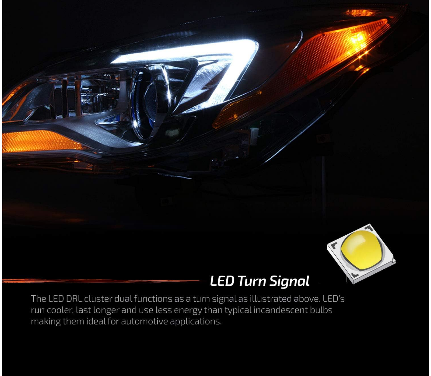
Figure 4: The LED Turn Signal activated, demonstrating its bright and clear indication for turns or lane changes.
