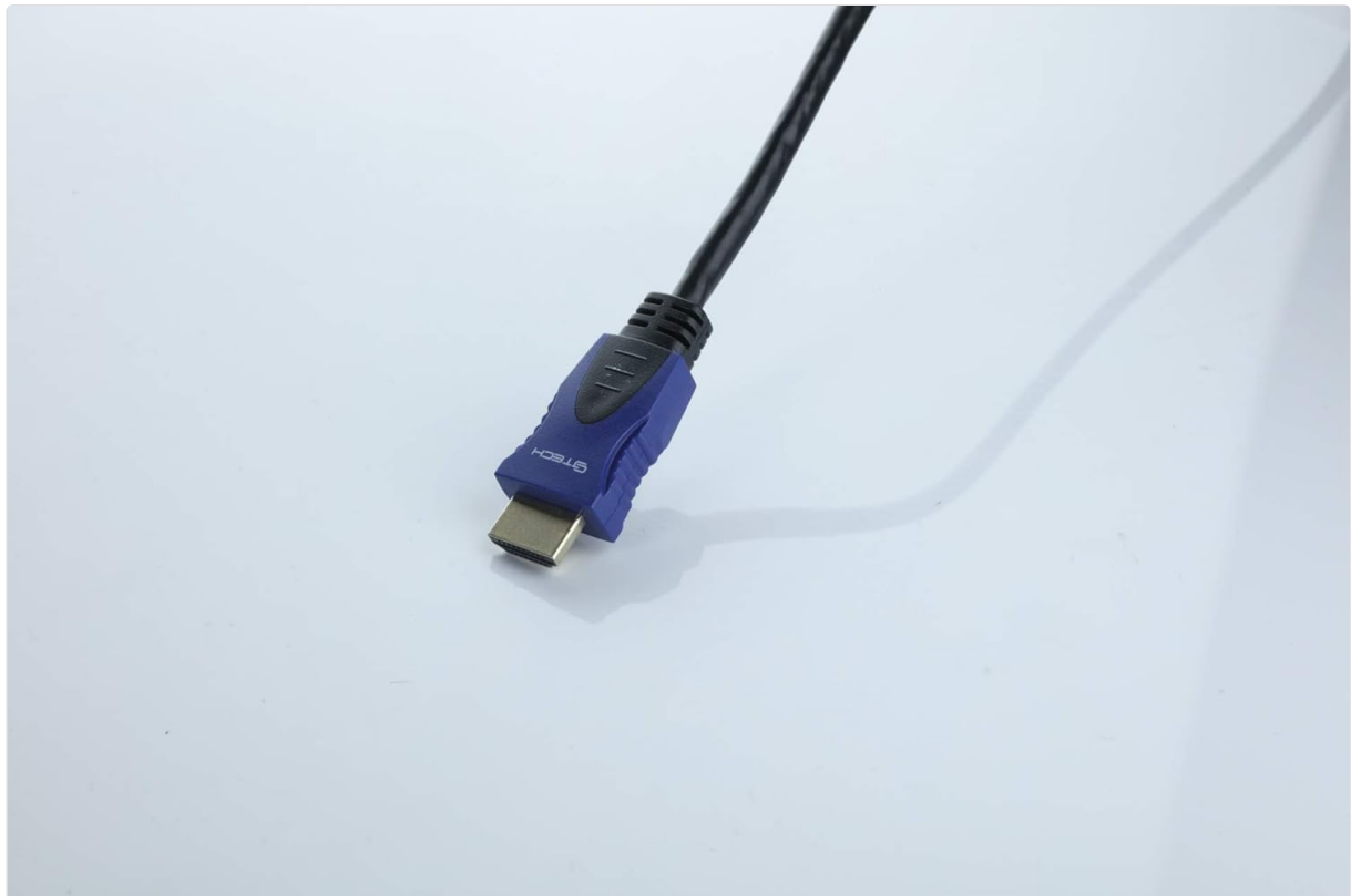
Figure 3: A close-up view of the HDMI connector, illustrating its design for secure connection.
