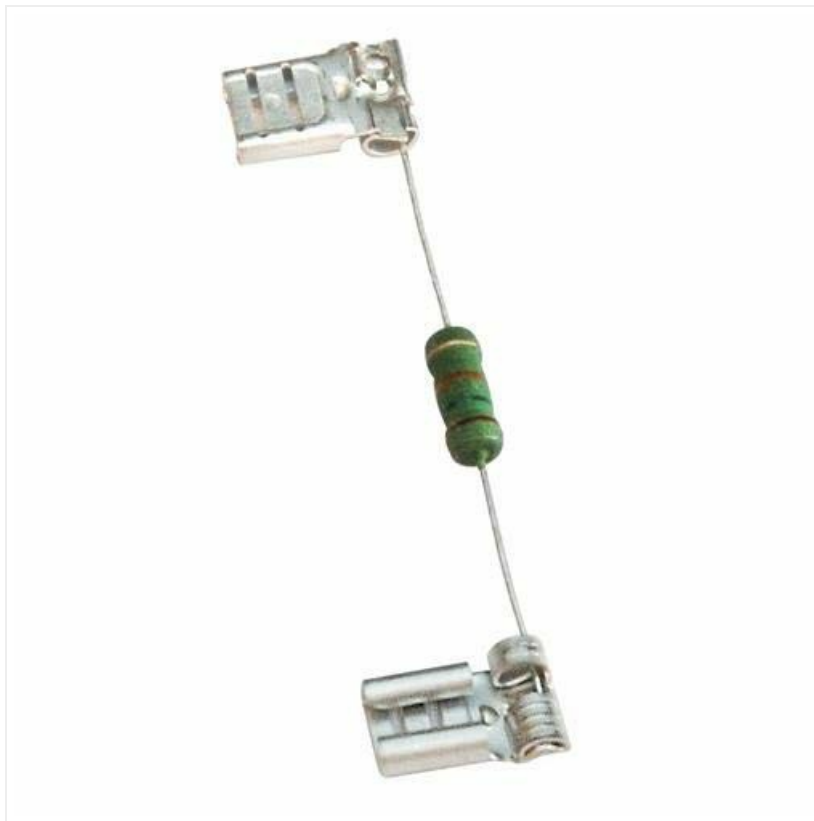
Image: The included 2-watt, 15K Ohm bleed resistor, which can be connected across the capacitor terminals.
